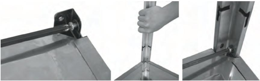
**STEP 6:** Unscrews 8pcs Standard Screws and Washers (BB) from top of tank housing assembly (K). Lift the assembled upper parts of heater and place them on the tank housing. Push support bar as photo showed and make sure each support bar inserts into slot. Fix at bottom position by using 8pcs standard screws and washers (BB).
