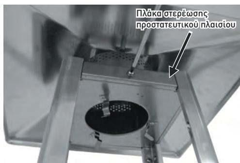
**ΒΗΜΑ 8:** Unload 4PCS Guard Fastening Plates by unscrewing 4PCS screws and washers from FLAME SCREEN (B).
