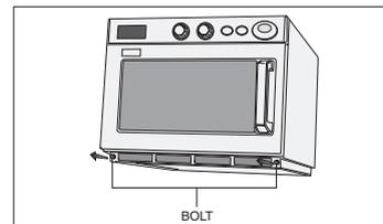
☑ If the Air Filter becomes clogged with debris, this will cause an overheating problem on the oven.
